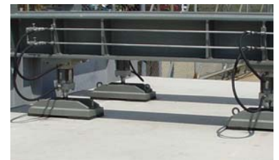
Dual Tandem Axle Pattern Loading on Actual Module
